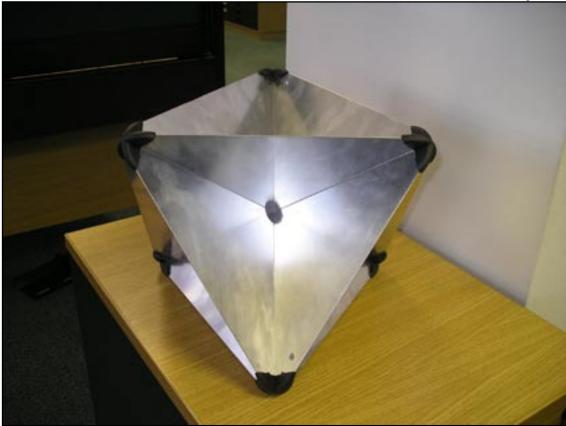
Octrahedral type radar reflector ("catch rain" position)
