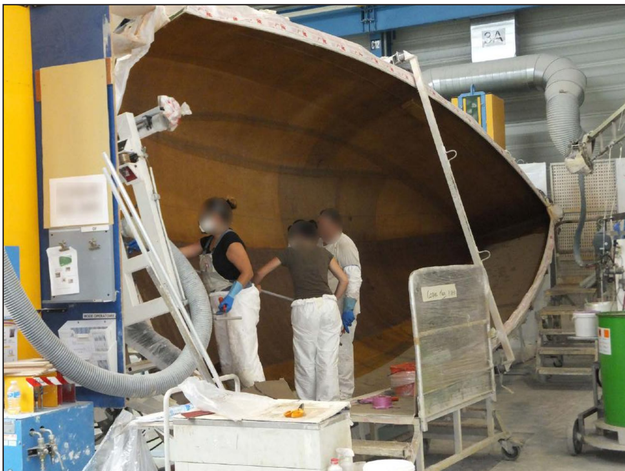
Figure 11: Hull being layed up in Beneteau's manufacturing facility (not a First 40.7)
