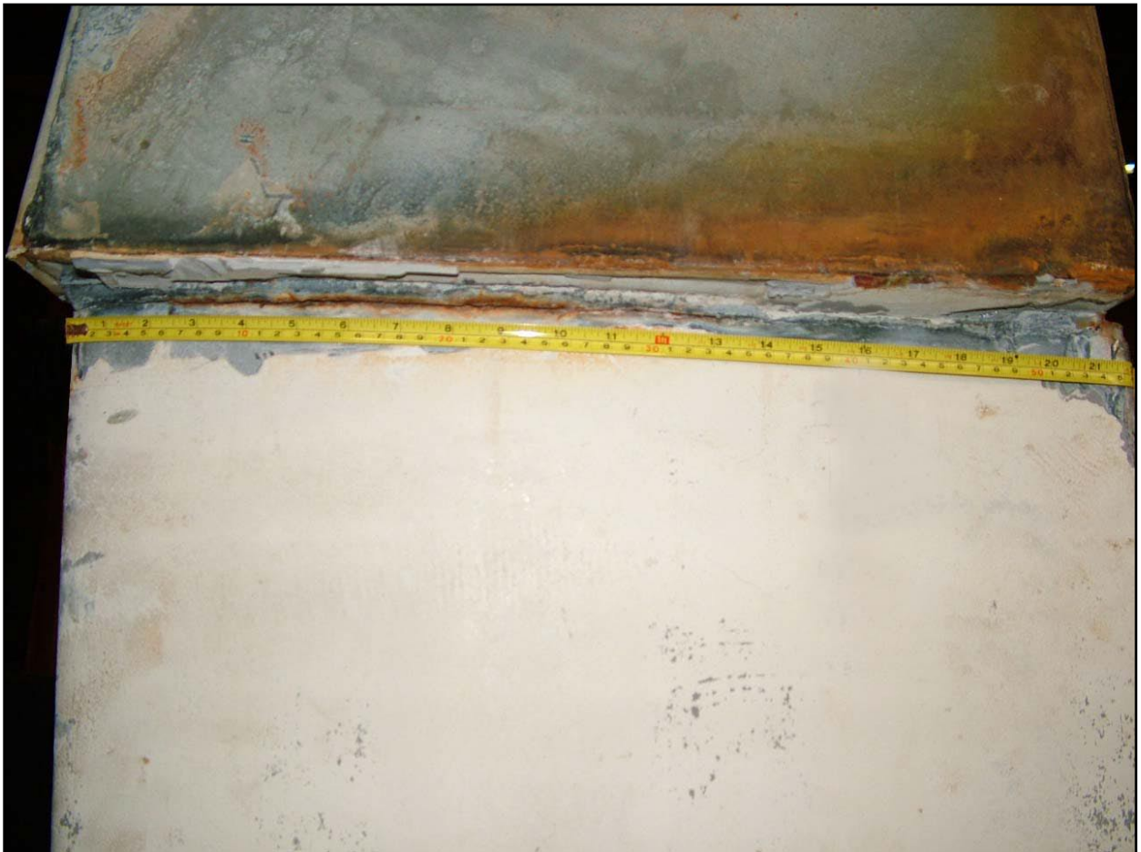
Fracture of the port side of the keel fitted to Who Cares
