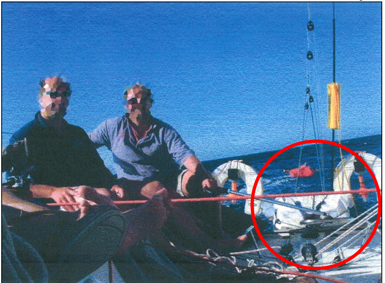
Position of liferaft and securing arrangement
