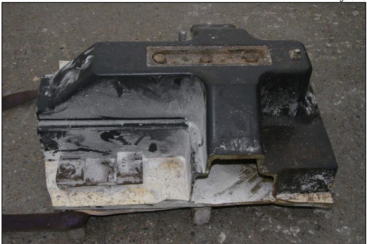
Removed keel remains and supporting structure
