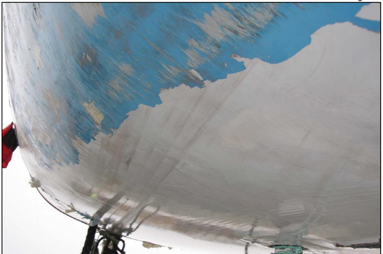
Paint and scratch marks on starboard side
