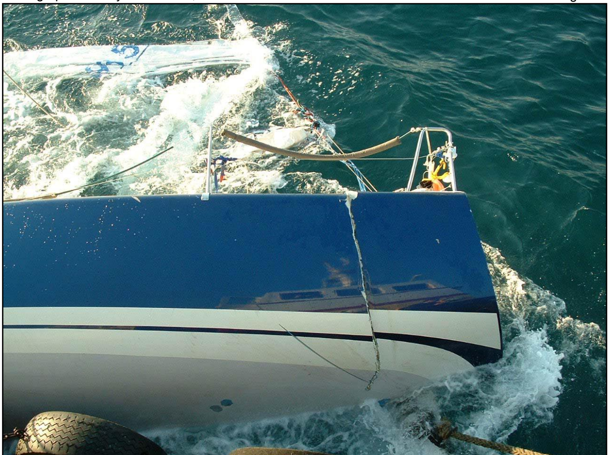
Rope damage to hull under port side of cockpit
