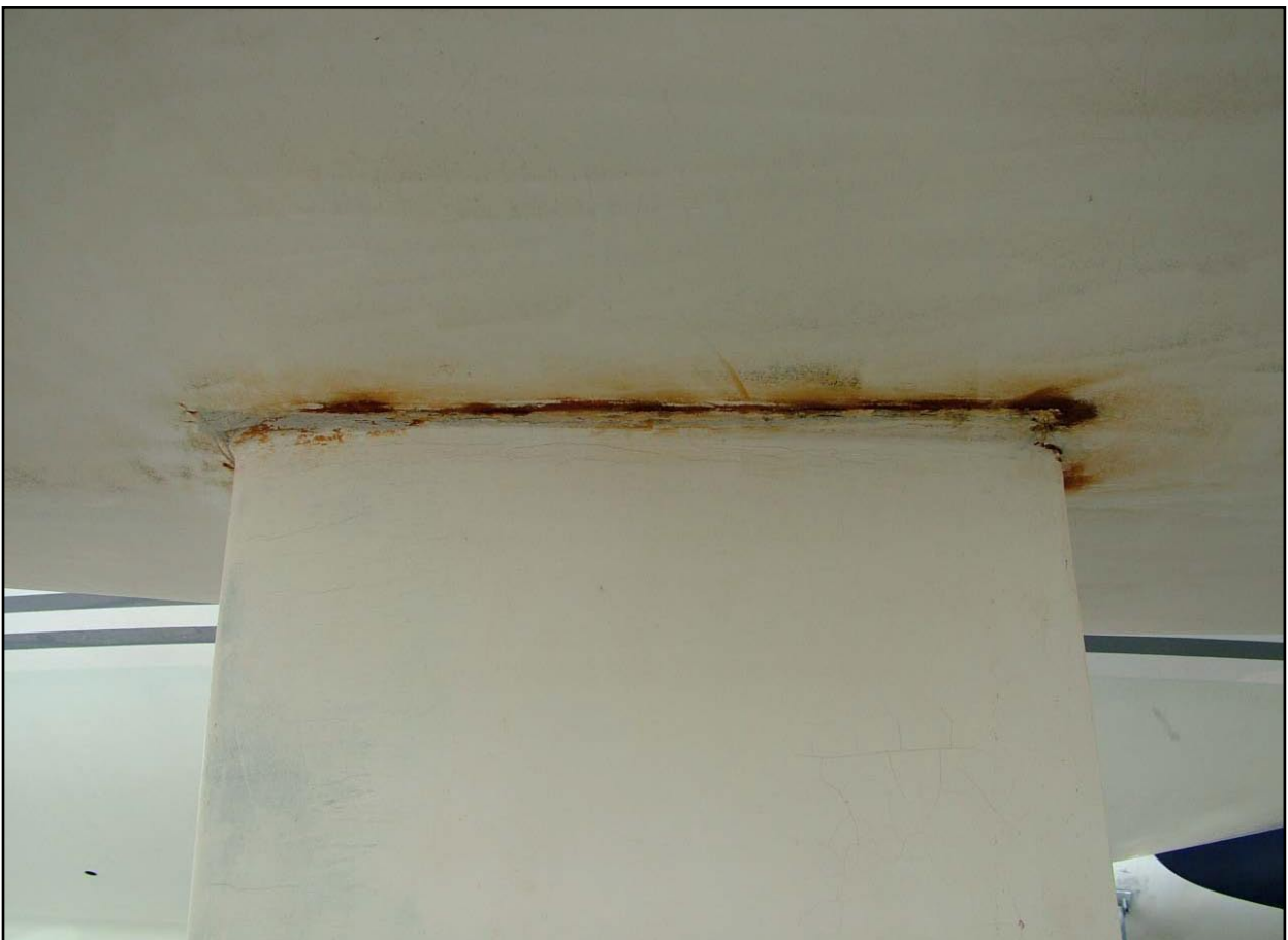
Keel of Mad Max showing cracking of the epoxy fillers and anti-fouling
