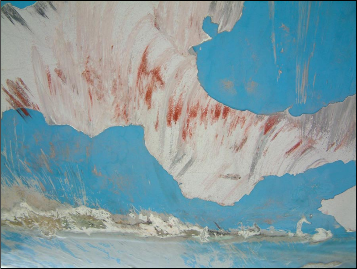
Paint and scratch marks on port side
